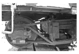
The other truck, further from the brake wheel, was a "winged" truck with extensions on the truck frame to hold the cross member which held the brake shoes, see below.
