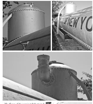
The flange of the vent is tightly riveted to the side of the dome. The rivets are much smaller in diameter than those used on the side and ends of the car too.
