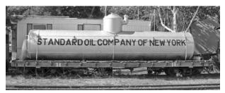
Car 22 at the Maine Narrow Gauge Museum was repainted into the Silver tank with the black Standard Oil lettering. It was painted with the number 14 on the flat car during our photography sessions which is incorrect as car 14 carried the larger tank which was made from individual panels which were riveted together.
