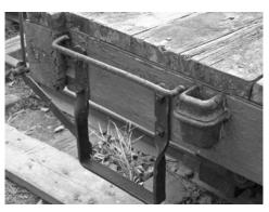
Each end of the flat car has an end step and a grab iron. The grab iron is wider than the end step.
