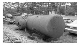
The No. 14 tank is laid on its side allowing photos of the underside of the tank with the dome cover off. The tank itself is very rusty having lain in the Edaville Junkyard for nearly 20 years before being transported to the Maine Narrow Gauge Museum.
