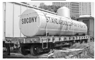
The brake wheel & staff normally would have been sticking up on this end of the car and placed just to the left of the draft gear.
